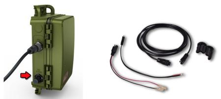
4. The external power cable includes F2-size spade connectors and ring terminals. Connect the cable to a 6 or 12-volt battery using one of the connectors provided. The SM4BAT FS provides protection against accidental reverse polarity connections.
