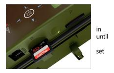
3. (Optional) To extend deployments, or to have a redundant card in case there is an issue with the first, insert a second SD memory card in the remaining slot.
