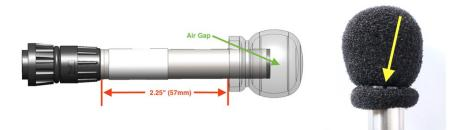
Do not handle or remove a wet windscreen as it is easy to accidentally squeeze the windscreen and push water into the end of the microphone.
