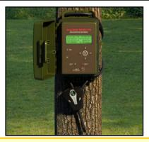
**NOTE**: Do not mount the recorder using a cable lock or other nonflexible cord to a growing tree. Circumferential growth could cause the cable to warp or break the recorder's mounting bracket. The tree won't like it either.
