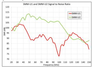
The higher signal-to-noise ratio means less noise from the microphone and higher signal. This allows the microphone to pick up fainter or more distant bats when recording. The SMM-U2 covers approximately 8 times as much airspace as the SMM-U1. The quieter recordings also result in cleaner, easier to analyze recordings that last longer and include more bat echolocation pulses. The microphone has a differential output which significantly reduces noise from electromagnetic sources.
