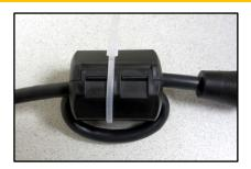
image shows the ferrite as shipped (right) and as installed (left).
