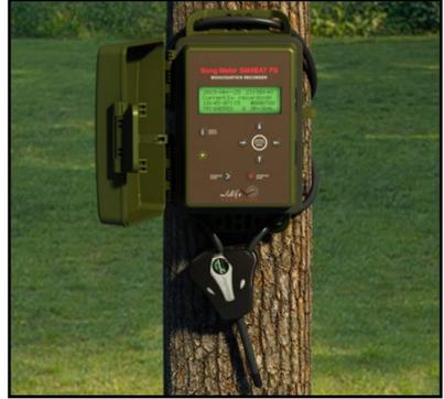
**NOTE:** Do not mount the recorder using a cable lock or other nonflexible cord to a growing tree. Circumferential growth could cause the cable to warp or break the recorder's mounting bracket. The tree won't like it either.
