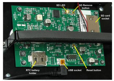
Here is an image showing the different parts inside the Roost Logger
